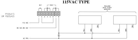
All circuits should be fused or protected by a circuit breaker (10Amp maximum)
